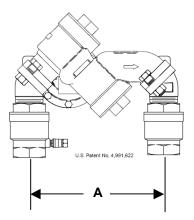
This variation in "A" has been found to be up to 1/8" for the 3/4"-1" sizes, and 1/4" for the 1-1/2"-2" sizes. The variation in centerline dimension has not been found to affect the overall performance of the assembly, however, it has been reported as a significant problem when a change-out of the body occurs in the field. If the inlet and outlet piping is fixed, a body being replaced with a different end-to-end centerline dimension will not fit.
